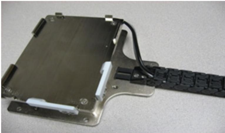
Figure 1: Cables routed and igus® cover installed
